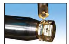
Drilling and milling a groove
