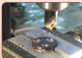
• Centering on Drilling Machine by PR Insert.
