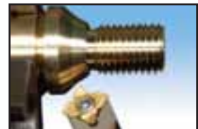
5 Taper turning, external
