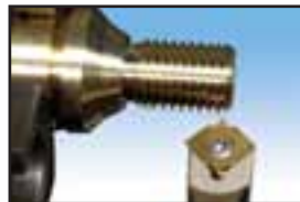
3 Thread turning, external
