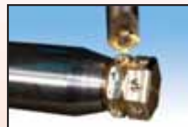
12 Drilling and milling a groove
